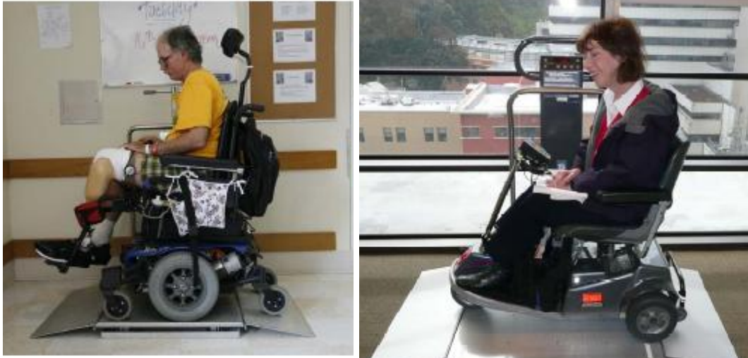
Figure 4. 14. (above left) standard stationary scale that may not accommodate a larger power wheelchair user (24" w x 30" l). Figure 4. 15. (above right) large-size (28" w x 32" l).
