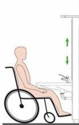
Figures 26 and 27: Accessible lavatory mirror If mirrors are to be used by both ambulatory people and wheelchair users, then they must be at least 74 in (1880 mm) high at their topmost edge.
